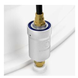
The wheel valve is a compressed air pressure-dependent valve that ensures that the tire is inflated at low pressures, and when it receives high compressed air pressure it switches over so that the tire can deflate. To make filling as quick as possible, you can work with two preset pressures: 4 bar or 6.5 bar. The higher filling pressure can easily save you 20 seconds of tire inflating time.
