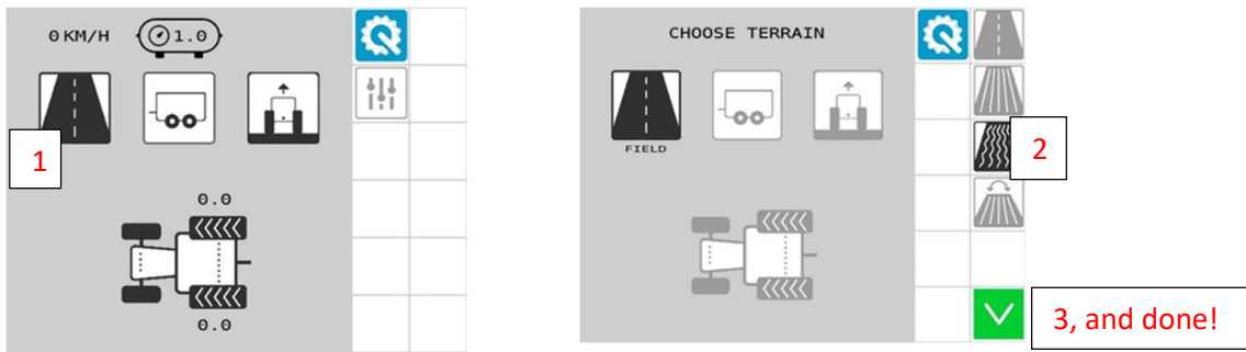
Example of choosing tire pressures for an extremely wet field.
